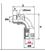
"EASY-ENTRY" 90° PLASTIC FITTINGS WITH ROTATING METAL THREAD IP 68/IP 69K (PG THREAD)
