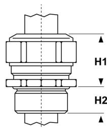
**"PROGRESS" A4 STAINLESS STEEL CABLE GLANDS FOR HIGH TEMPERATURES - "AGRO" SERIES (PG THREAD)**
