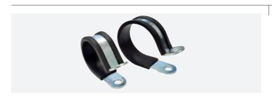
SKM/SKM-E: **Galvanized steel cable clamps with rubber or EPDM lining.**Flame-retardant and self-extinguishing, they are suitable for fixing pipes and cable bundles. The rubber lining offer protection, anti-vibration function, excellent electrical insulation and resistance to ozone, UV rays and atmospheric agents (EPDM).
