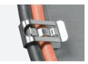
CMF-IN: Clips for max 2 cables, with cables inside the frame. Clips oriented so that the cables are hidden inside the photovoltaic module frame. Suitable for cables with diameter 5.1 - 8.4 mm each, for frame thickness 1.4 - 3.2 mm.
