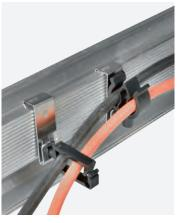
Cable holders for modular clips, available in rectangular shape (also 90°), in round shape with locking closure and in Helios shape (also 90°). They can be mounted to the CMF-CM and CPS-CM modular clips and allow you to secure and organize cables and cable bundles of various sizes.
