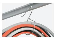
SUNHANGERS: **Stainless steel hangers**. Made of corrosion resistant 304 stainless steel, these innovative products can be hung from structures or hooked into holes to support and organize bundles of cables and hoses. They can be easily closed with a simple pressure and can be reopened for maintenance or replacements. They are available with horizontal or perpendicular (90°) cable orientation and with PVC coating for additional protection to cables in harsh environments.
