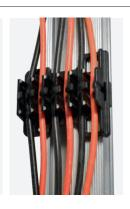
MAXRUNNER: Cable holding plates for screw mounting or stainless steel mounting clip. Designed to organize cables safely with locking tabs that ensure a firm hold. They can hold up to 12 cables with diameter 5.2 - 7.2 mm each. The stainless steel clip plate allows mounting on structural profiles with edge width 1.5 - 6.4 mm. Made of UL94-V0 PPE + PS, they offer excellent resistance to outdoor exposure.
