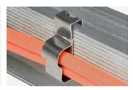
CPS-2C: **Clips for max 2 cables**. Clips suitable for micro-inverter cables with diameter 7.6 - 12 mm each, for profile edge width 2 - 9.7 mm.
